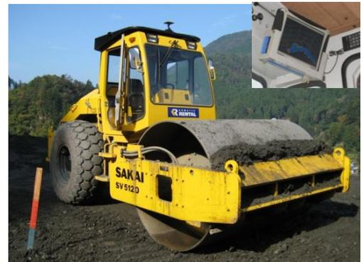
Figure 1. Compaction control system by RTK positioning
